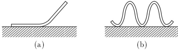
Fig.1 Identifiable contact states of edge
