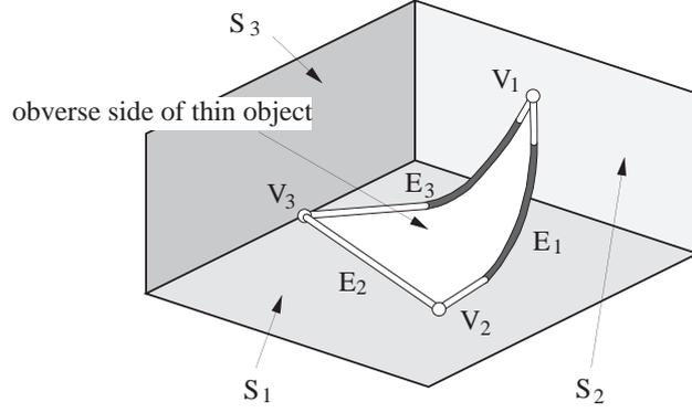
Fig.3 Example of contact state with respect to multiple environmental surfaces
