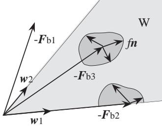
Figure 1: Condition for bounded force closure
