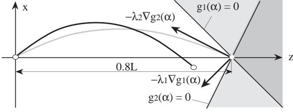
Figure 4: 2D-deformation of a linear object corresponding to inequality conditions
