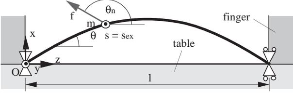
Figure 5: 2D-deformation of a linear object imposed an external force and moment
